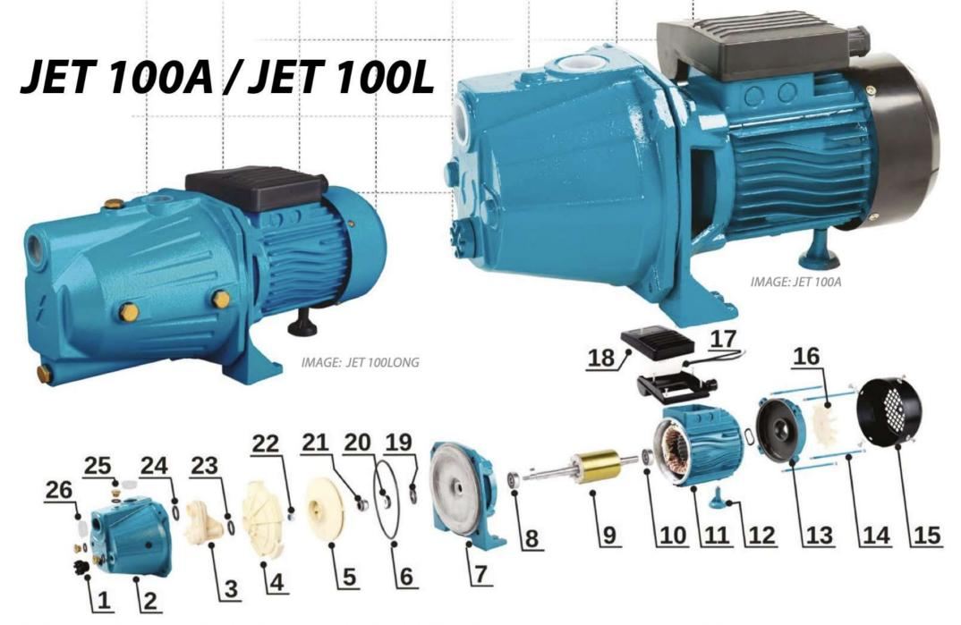
Single-stage self-priming centrifugal surface pump equipped with the Venturi tube system for increased suction capacity, designed for pumping of clean cold water from own intakes and for increasing pressure. The pump body is made of durable cast iron, and the pump motor is provided with thermal protection. The pump has a power cable with a plug. The pump is available with accessories or
